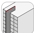
water stop with coating at the splice
