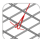
Preformed rods with loop - no welding required
