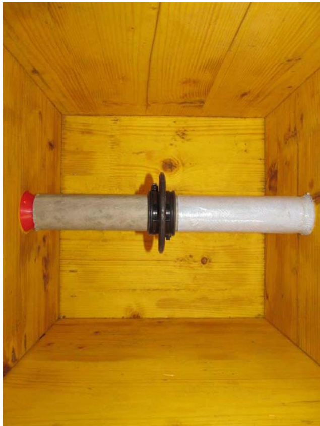
Figure 4: Fibre cement distance tube enveloped in a water-permeable sleeve on one side up to the sealing collar to ensure trans- portation of the water
