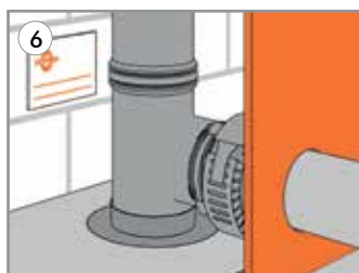
6 Panelling / encasing of the seal Zero clearance of the casing to the firestop collar or connector permitted. Complete the fire protection sign and attach it so it is visible when the casing is removed. Complete the conformity attestation and give to the building owner.
