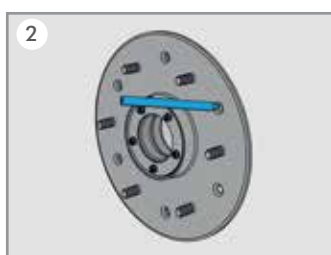
2 Mark the rawplug holes, drill holes and insert the rawplugs.
