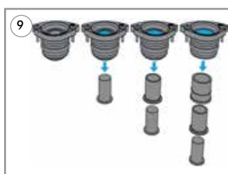
9 Removed the dummy stoppers from the seal unit and adapt the module seal in accordance with the water service line diameter.
