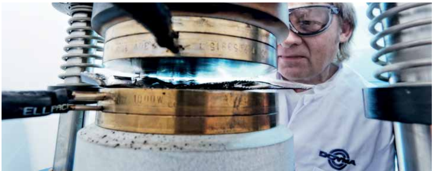
Inflation pressure testing for intumescent material
